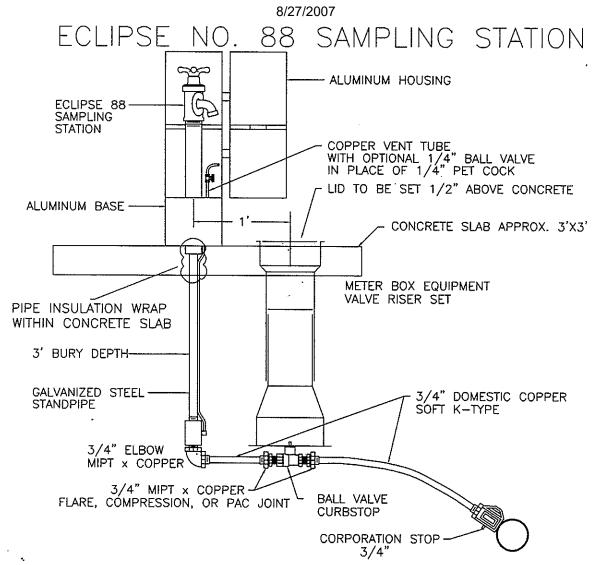
Sampling Stations shall be a 3' bury, with a 3/4" FIP inlet, and a (3/4)" hose or unthreaded) nozzle.
