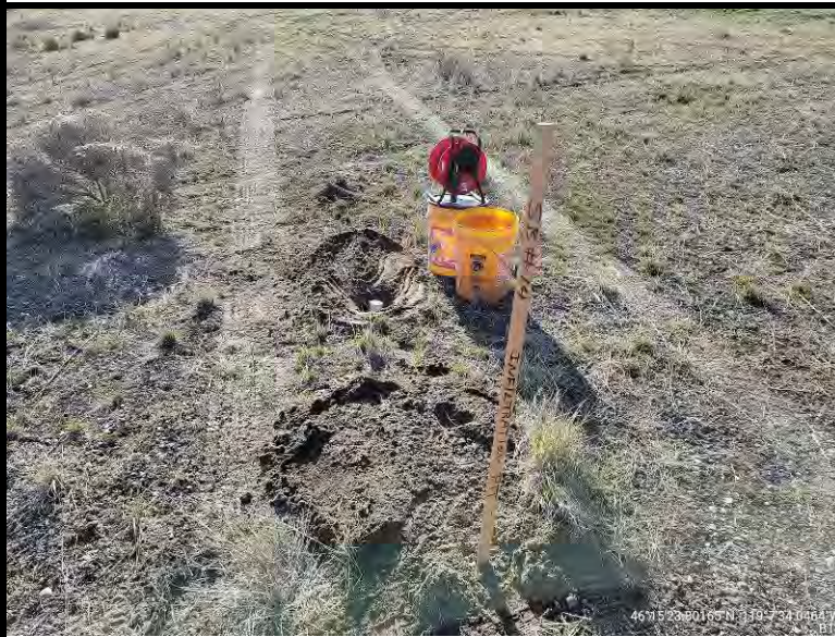
View of infiltration test equipment at Boring B-14
