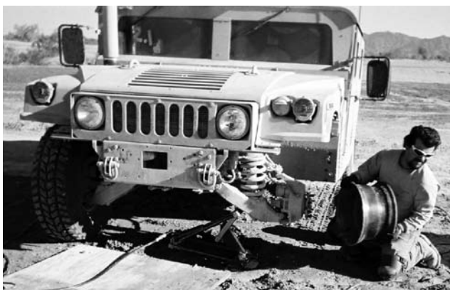
The jack passed tests that simulated conditions in Iraq.
