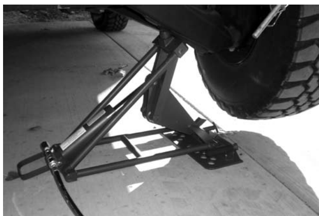
The jack takes one person just three minutes to lift a Humvee.
